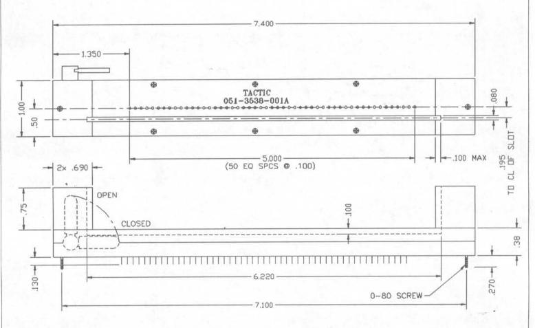
This series is designed for long in-line packages that are wider than two rows, with either square or staggered device lead patterns.
