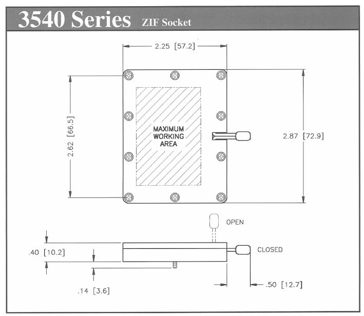
This series is designed for any number of pinned packages with 1,2,3 or 4 sides, and in-line, square, or round patterns.
