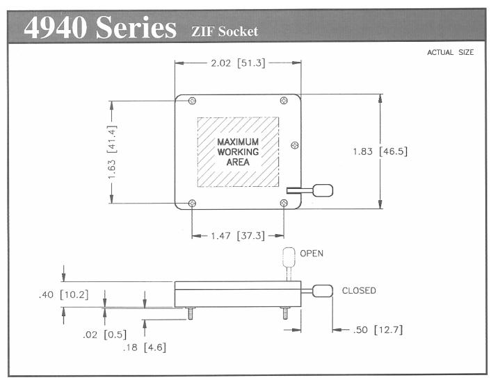
This series is identical to 3540 series with the exception of the overall size. Maximum working area: 1.3" x 1.1" Minimum lead length: .100"
